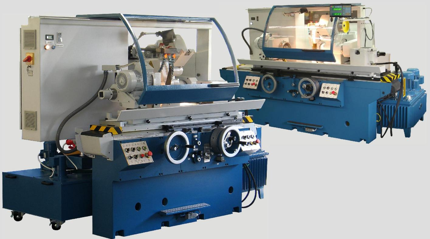
Universal grinder for rollers RUP-280 is appropriate for grinding internal and external rotary surfaces and also for grinding flat fronts of different workpieces and flanges.
